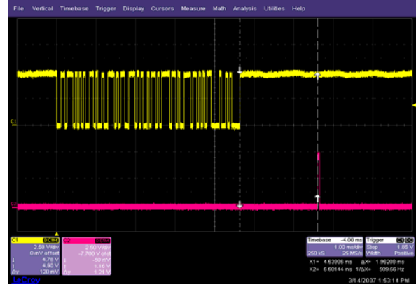
Fig. 6 Screenshot of oscilloscope - delay for execution 1.96ms
